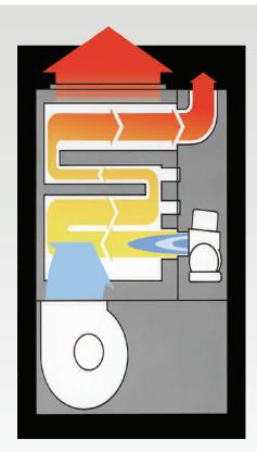
The combustion/heat exchanger combination is a Bryant® exclusive. This unique component quickly and efficiently converts oil to heat so your family can relax in the soothing warmth of home.
